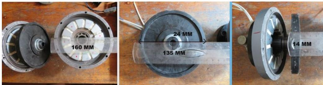
The **1** has **2** ball bearings on its axis and its magnetic segments, with a total weight of 2.57 kg, face the coil at 2 mm each.
